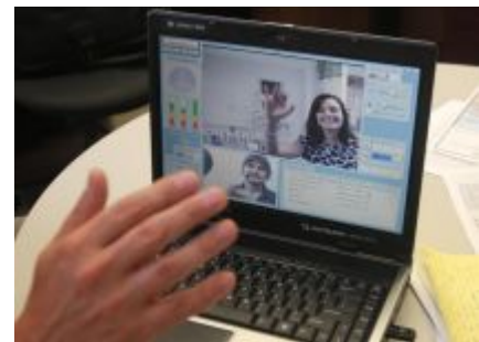
CONTROL CENTER: Remote-presence robots are controlled with a wireless-equipped laptop and special joystick. EDGAR can take pictures, print prescriptions and hook into machines to transmit medical data from the hospital to a consultant in a different room or a thousand miles away. - The Observer/CHRIS BAXTER
